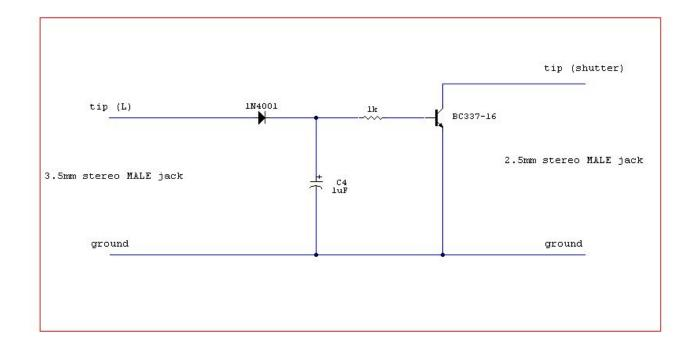
This is basically a 2 wire cable terminated at each side by a MALE stereo jack of two different sizes, 3.5mm on the computer side, 2.5mm on the camera side, with 4 electronic components in between: if you are able to work with SMD components like I do, you can even implement the whole circuit in the jacks shells, ending up in a neat, simple looking cable...
