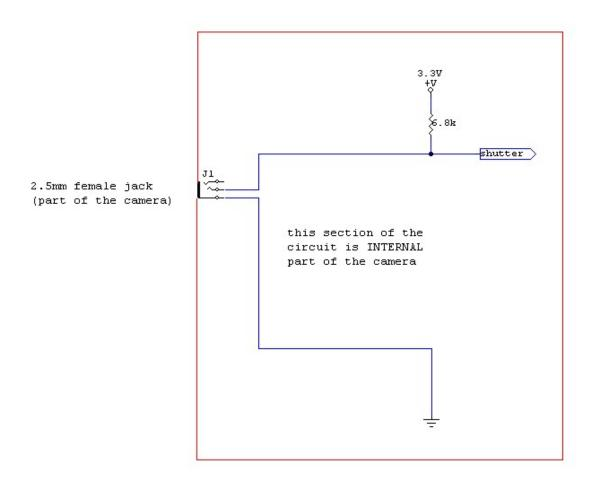
This is the equivalent circuit of the shutter sensing system INTERNAL at the camera: Is important to see the 6.8k Ohm resistor pulling to 3.3V the tip contact of the female jack, because this is a wise method to drive to ground the "shutter" labeled point (camera logic checks this to decide the shutter status), preventing 3.3V camera supply to short (that is the reason why you could even use a mechanical switch or whatever similar to fire the camera safely).
